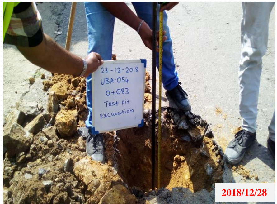
Test Pit Excavation UBA 054 CH- 0+083
